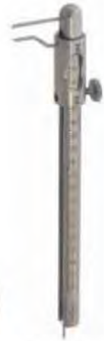
DM-1454 Gauge for measuring distances (0 - 90 mm),
